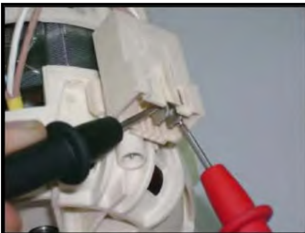
Measurement of the primary windings of the washing pump
